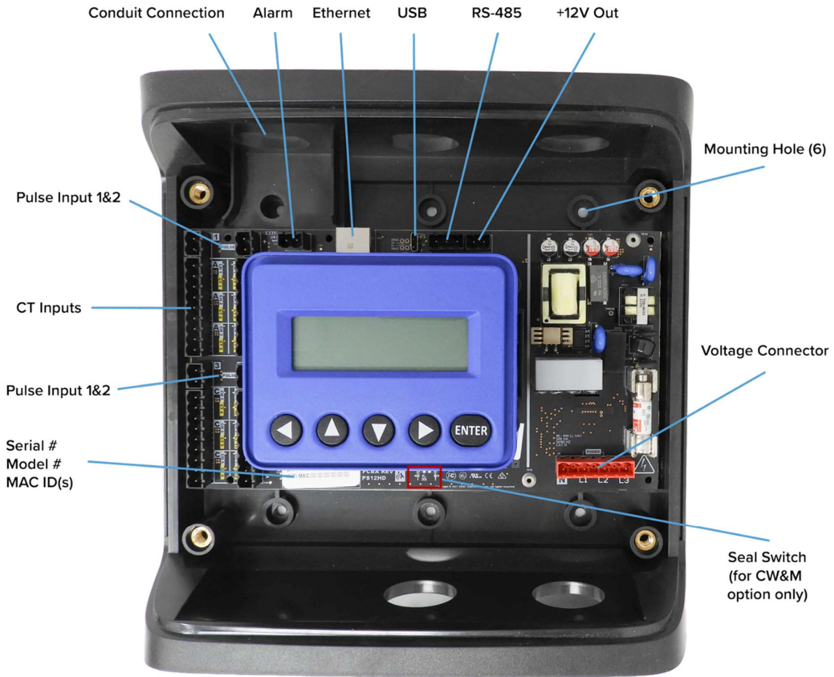
PS12HD (Enclosure with cover removed)
