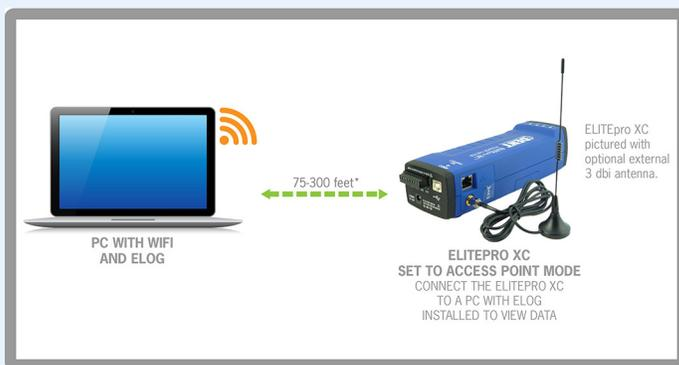
Access Point mode sets the ELITEpro XC as an access point. View real-time data on a wi-fi-enabled laptop running ELOG software.
