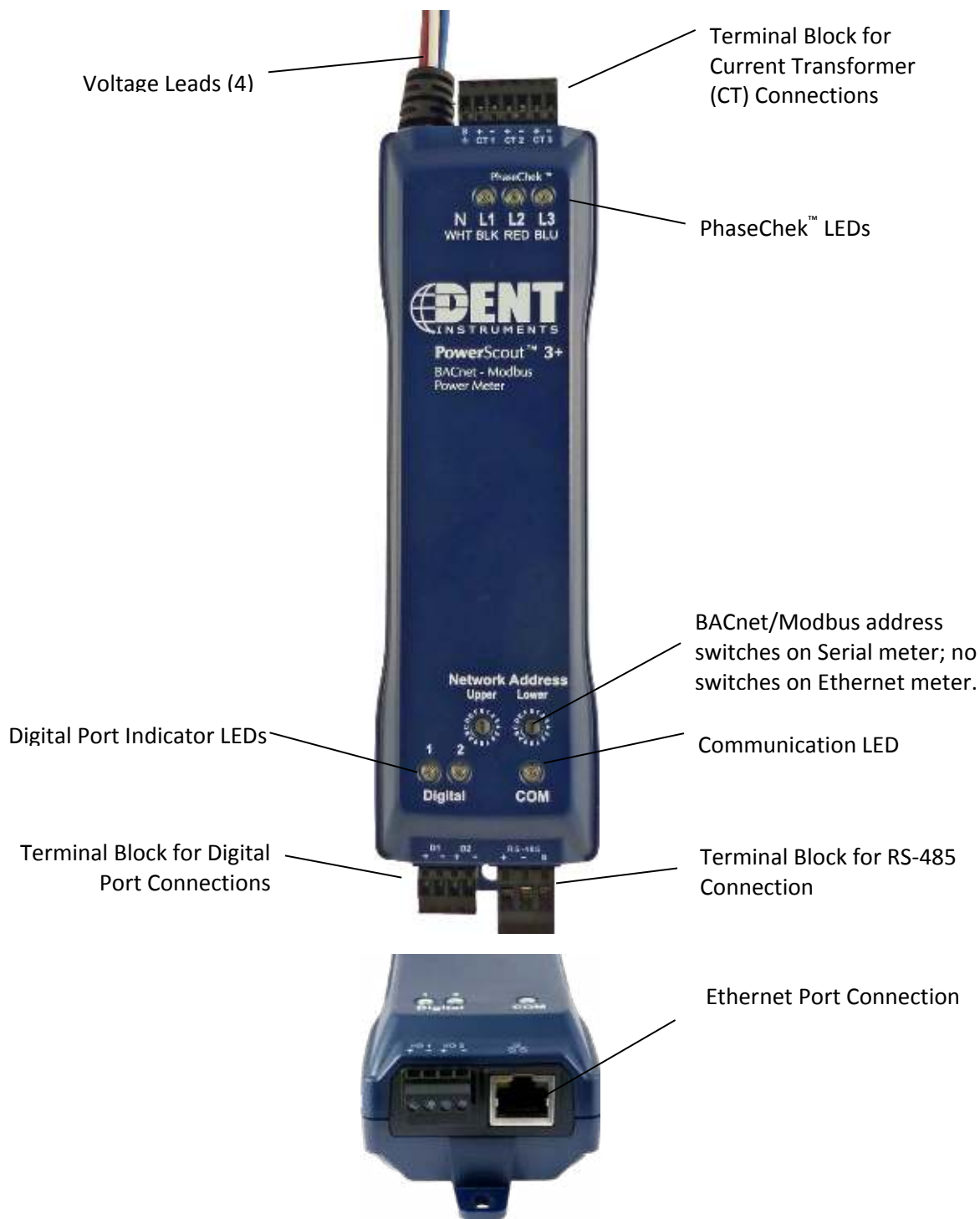
Figure II-3: PowerScout 3 Plus Layout—US voltage wire colors shown
