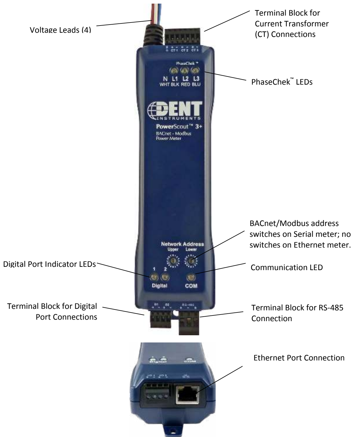
Figure II-3: PowerScout 3 Plus Layout—US voltage wire colors shown
