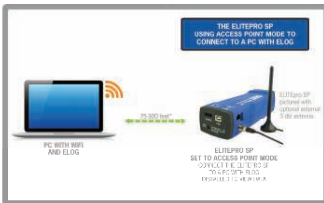
Access Point Mode using ELOG to interface with an ELITEpro SP with Wi-Fi.
