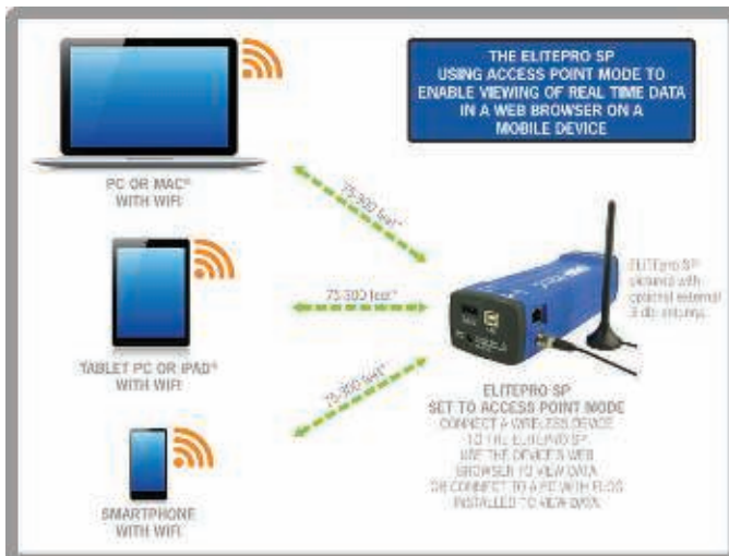
Access Point Mode using a web browser to interface with an ELITEpro SP with Wi-Fi.
