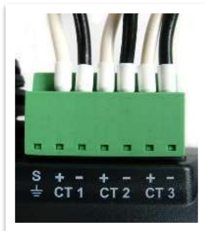
Photo 4: Connect White Wire to Positive Terminal. Connect Black Wire to Negative Terminal.
