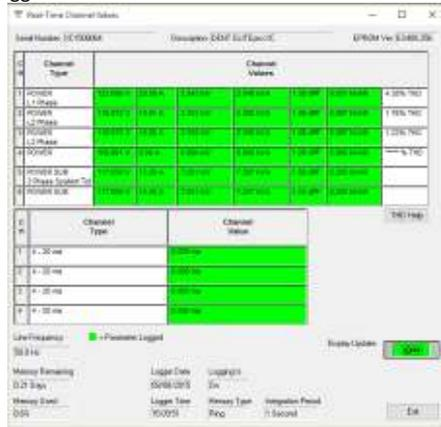
Allow the logger to collect several minutes of data. Collected data can be saved as an .elog file on the hard drive.
