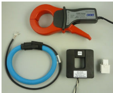
Figure 2: A wide range of current transformers (CTs) can be used, including (clockwise from top) 1000A Clamp-On, 50A Mini Hinged, 200A Split Core, and 16" RoCoil (Rogowski) CTs.
