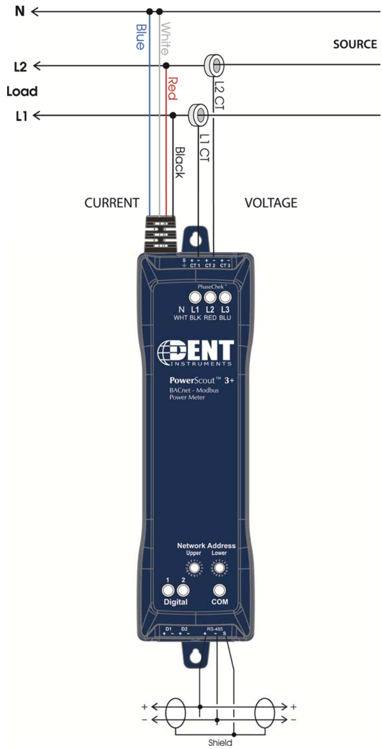
Figure IV-2: Single Phase, Three Wire
