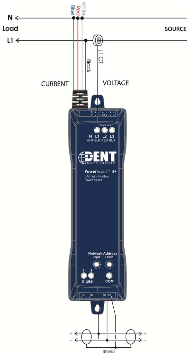
Figure IV-1: Single Phase, Two Wire
