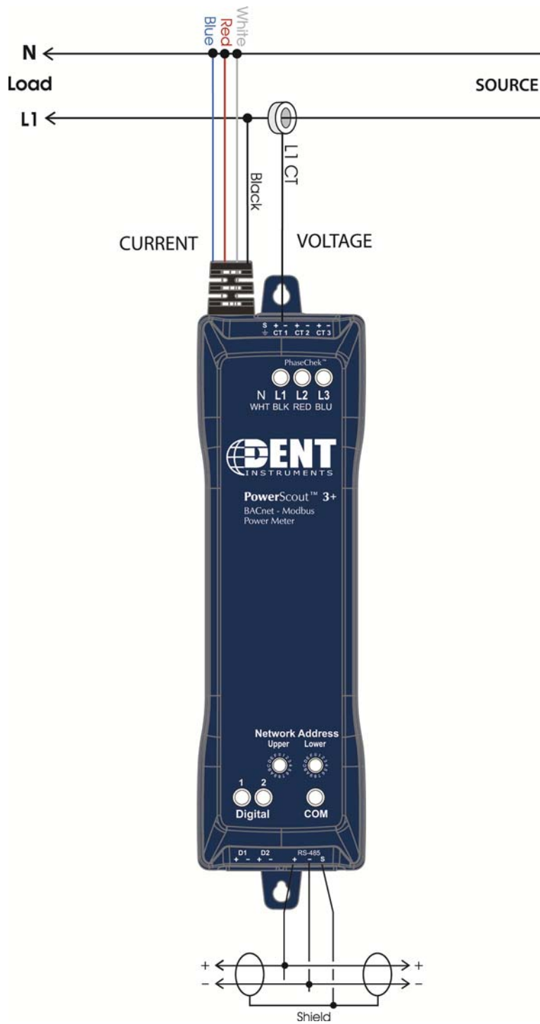
Figure IV-1: Single Phase, Two Wire
